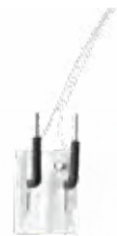
L-shaped (short) Electrode for field stimulation of mounted muscle ring preparations (eg aorta and bladder rings).
