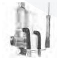
L-shaped Electrode (short/reverse) for field stimulation of mounted muscle ring preparations (eg aorta and bladder rings).
